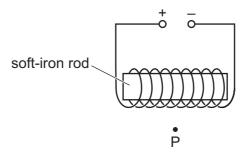
A small compass needle is placed at point P.
