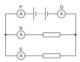
Which two ammeters read the largest current?
