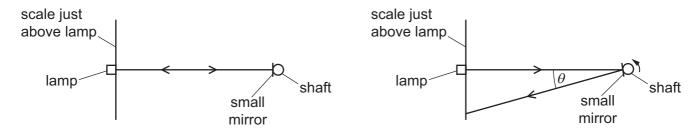
The beam from the lamp reflects from the mirror to give a small spot of light on a scale placed just above the lamp. The shaft and mirror rotate through 1°. The spot of light moves along the scale.
